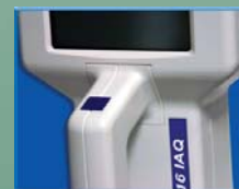
One-handed Operation with Start & Stop on Handle
