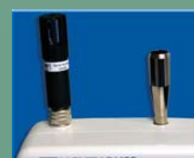
Removable Temp / RH and Isokinetic Probes
